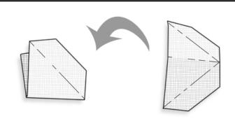
3. Fold the scored lines to obtain flexible axes. Fold the mechanism in two.
